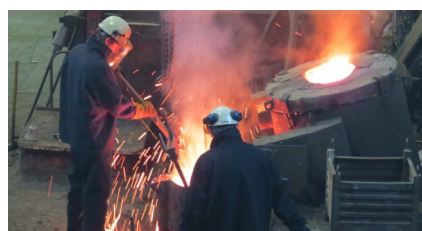
A bell being cast at Taylor's bell-foundry
